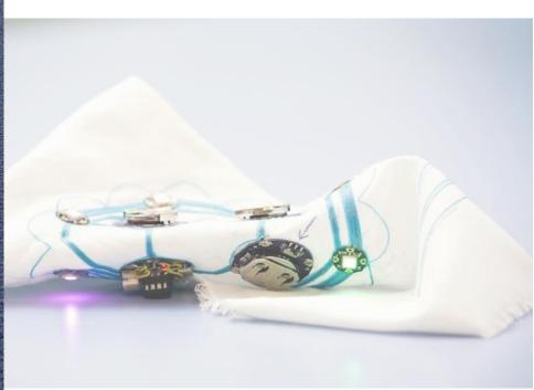
Embedding of electric conductive yarns by 3D printing
